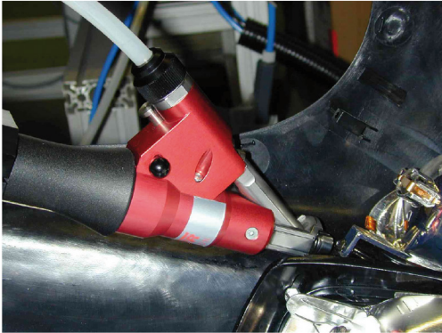
Fitting headlights in motor scooter fairings
