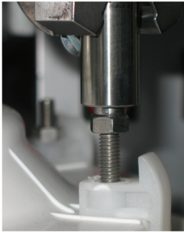
Fitting nut (screwdriver with vacuum tool)
