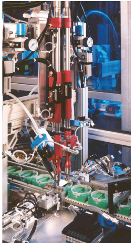
Inserting thread-forming screws into plastic rings for the electro-industry
